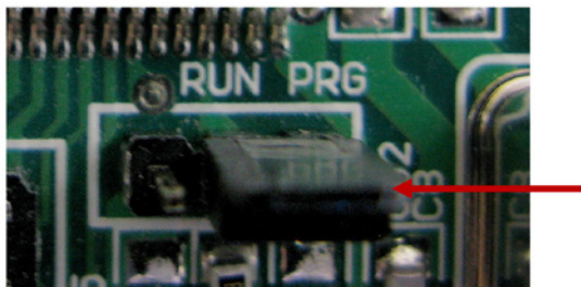
Figure 26: Programming Jumper in the PRG Position
