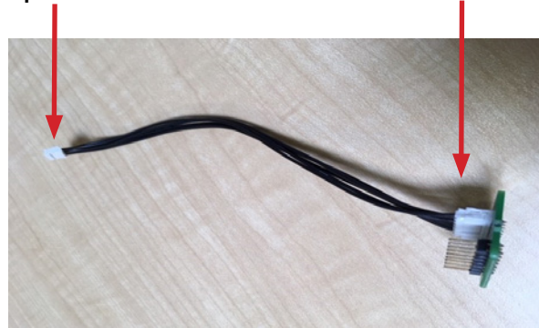
Figure 7: Inserting the Renesas E2 Lite 14-Pin Ribbon Cable to the PCB Board of the Interface Cable
